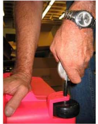
10- REPLACE PIN WITH "7047 Rev B" PIN
